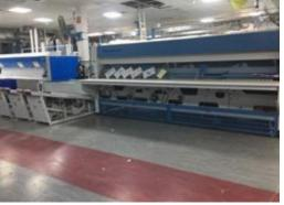
A new ironer was installed in the laundry, which can now cater for four hotels and Wild Wadi Waterpark. The overall cost per kg of ironed linen has been reduced due to more efficient energy consumption and there has been a 40% reduction in steam consumption compared to the original ironer. The cost saving when the hotels are at 70% occupancy is 65,000 AED/month - equates to a ROI of 37 months.
